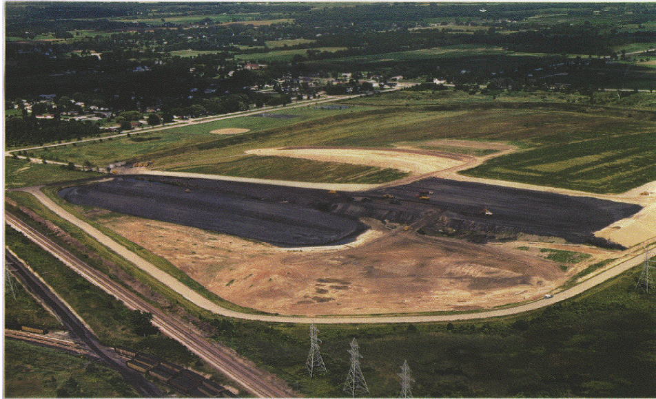
Figure 1-4: This 170-acre coal ash landfill is located in Oak Creek, Wisconsin, where over 3,700,000 cubic yards of coal ash are stored.
